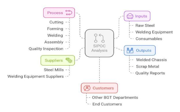
The chassis fabrication process is illustrated in Figure 3. The process begins with the receipt of raw materials and proceeds through cutting, welding, assembly, and quality control before the finished chassis is prepared for shipping.
